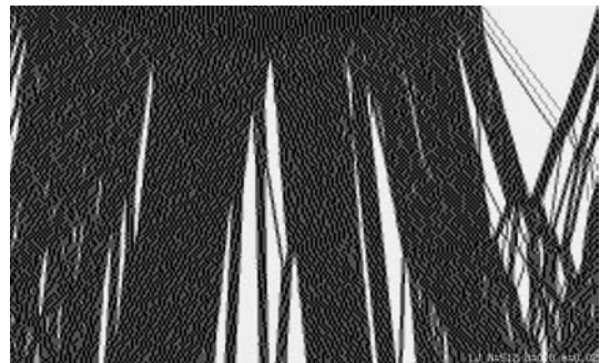
Fig. 4. The evolution of the particle density for d = 0.8 , N = 512 and e = 0.02 . Along the horizontal direction a black pixel is drawn at each particle location. Time increases downwards.
